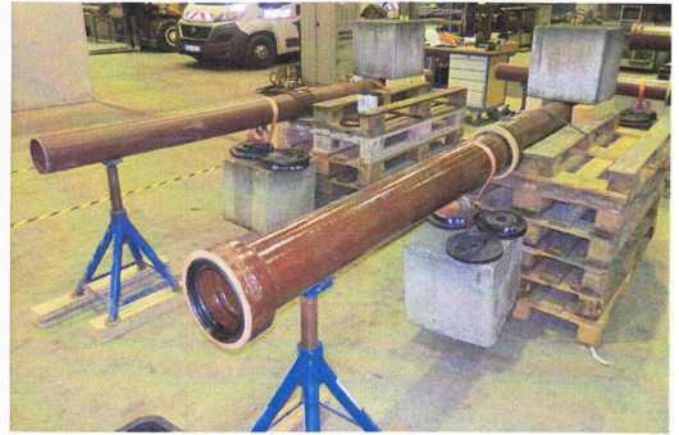
Figure 4: Shear load influence on trial segments 1 and 2, DN 150
