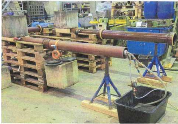
Figure 3: Leakage testing with shear load, Trial segment 1: PVC-PVC, DN150
