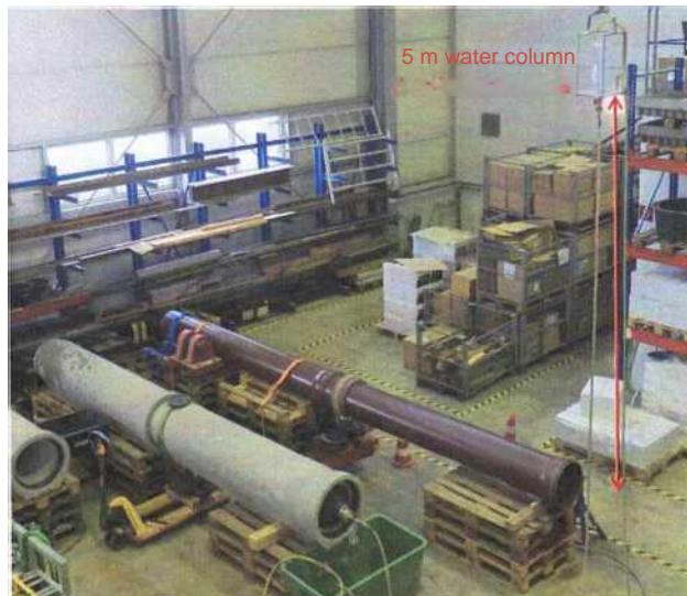
Figure 7: Leakage testing with shear load, trial segment 4: Concrete-concrete, DN 400
