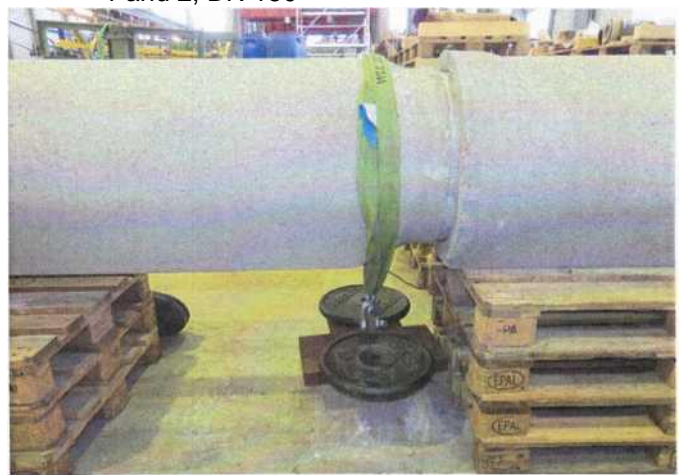
Figure 6: Shear load influence on trial segment 4: Concrete-concrete, DN 400
