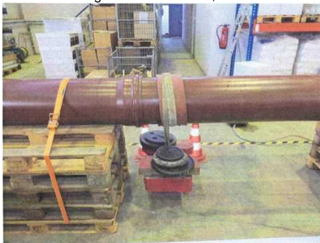
Figure 5: Shear load influence on trial segment 3: PCV-PVC, DN 400
