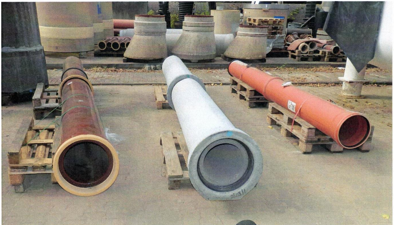
Figure 4: Test segment 1 (stoneware-stoneware), test segment 2 (concrete-concrete) and test segment 3 (PVC-PVC) DN 300
