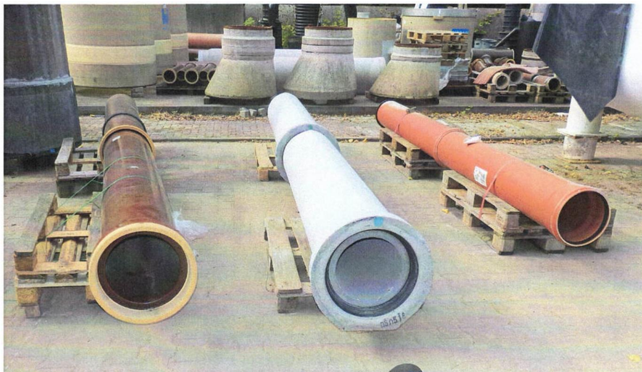
Figure 2: Test segment 1 (stoneware-stoneware), test segment 2 (concrete-concrete) and test segment 3 (PVC-PVC) DN 300
