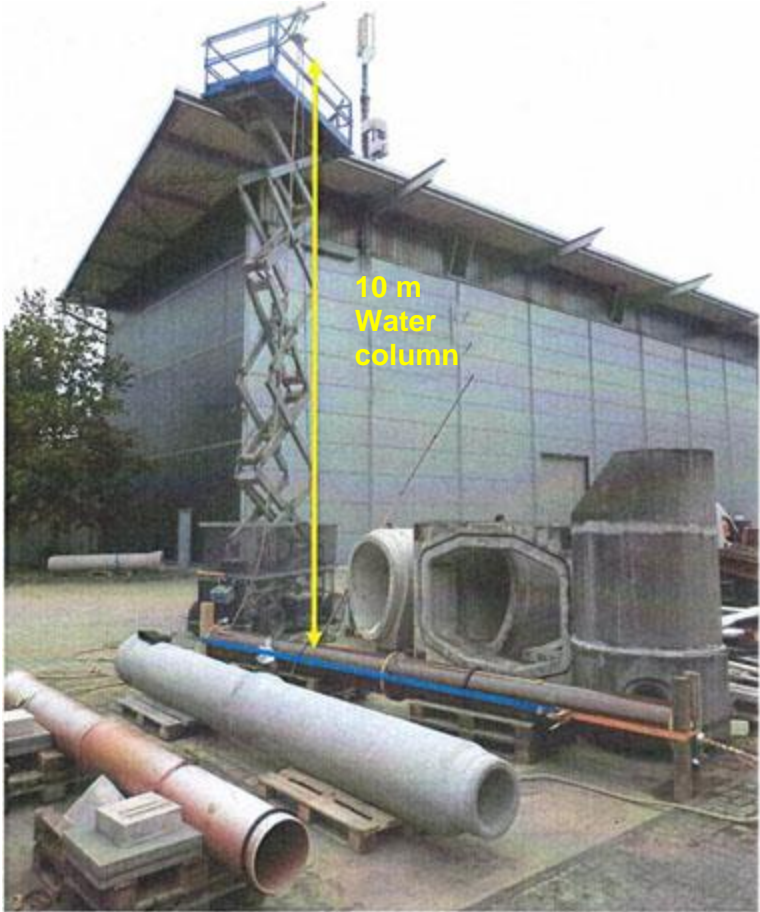
Figure 10: Test setup for the leakage test with 0.1 bar (10 m water column)
