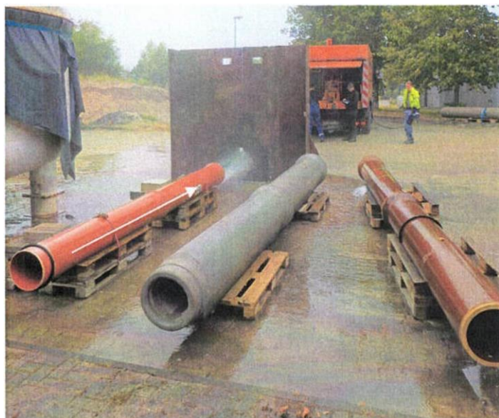
Figure 7: Trial implementation test segment 3 (Direction of flush in the direction of the arrow)
