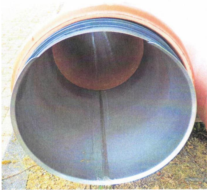
Figure 11: Circum-MINI (interior pipe collar DN 300 after 60 cycles)
