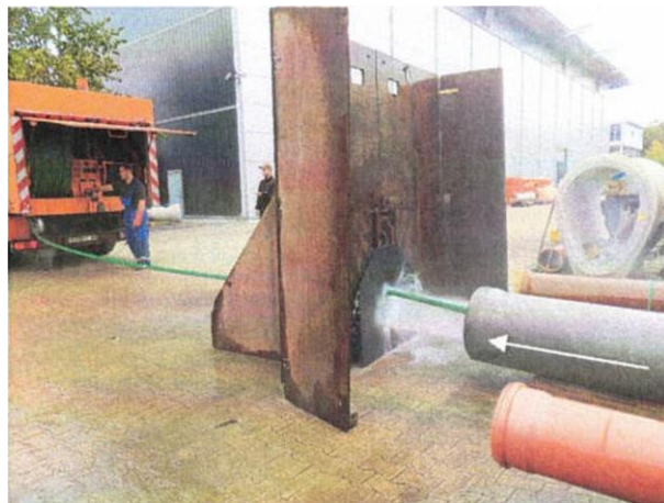
Figure 6: Trial implementation test segment 2 (direction of flush in the direction of the arrow)
